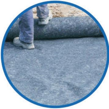
**NON-WOVEN GEOTEXTILE:** Permeable blankets of filaments or synthetic fibers randomly distributed, used for separation, filtering, drainage, protection and reinforcement.
